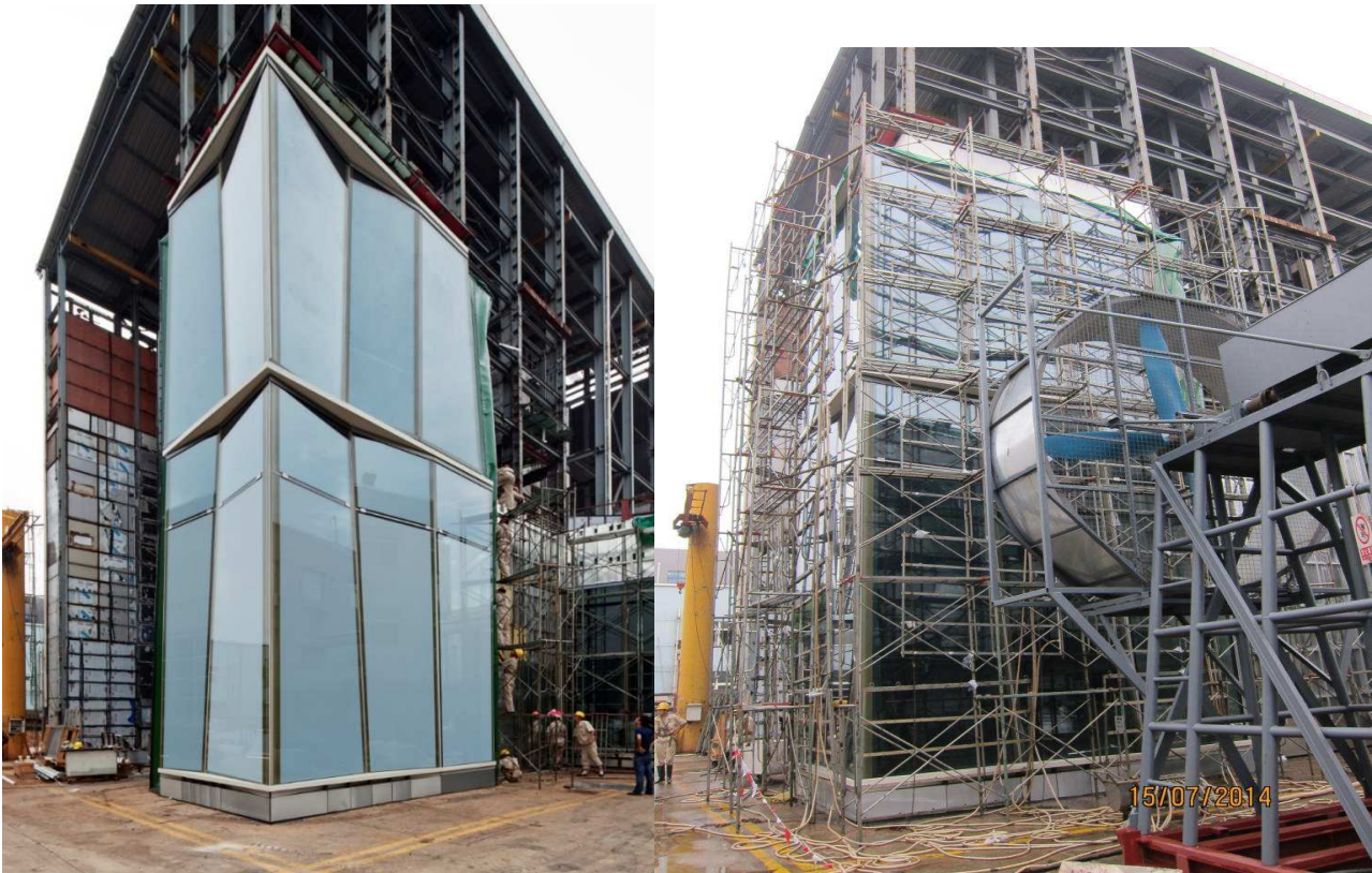
Figure 12 + 13: Test of the performance mock up done by the facade contractor yuanda
